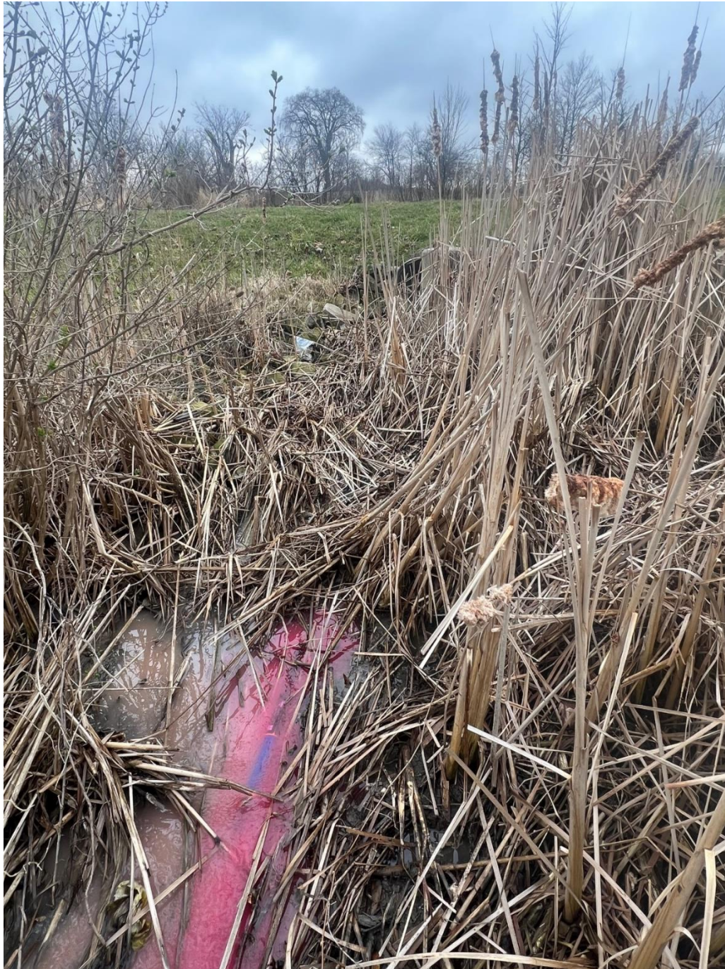
Photograph 6. Southwest view at 12:00 pm of the rhodamine dye within the watercourse flowing through Rock Street Park. This photograph is northeast of the newly identified “South Rock Street Park Spring” which is located on the channel-bottom, immediately north of the culvert passing under Townline Road, at the intersection with Rock Street. Dye was first observed emerging from “South Rock Street Park Spring” at 11:53 am, and following this observation, the rhodamine sonde installed at “Rock Street Park Spring” was moved to this location (Photograph was taken on April 4, 2024).
