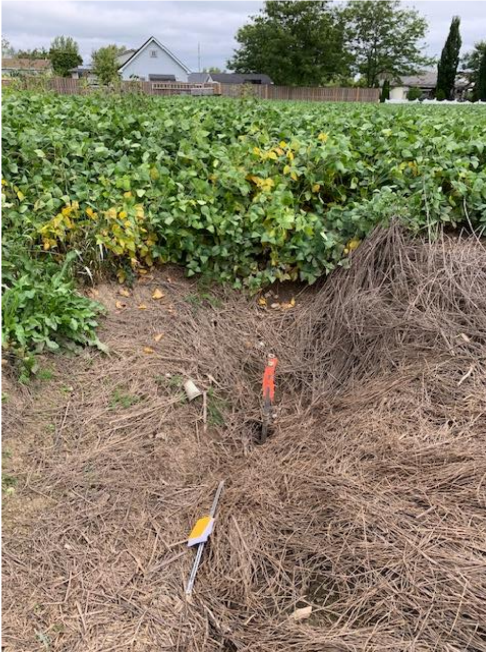
Photograph 1. Northward view of SH-SE-1 with Drive Point installed (contains water level datalogger) and flagged with orange tape (Photograph as taken on September 13, 2023).
