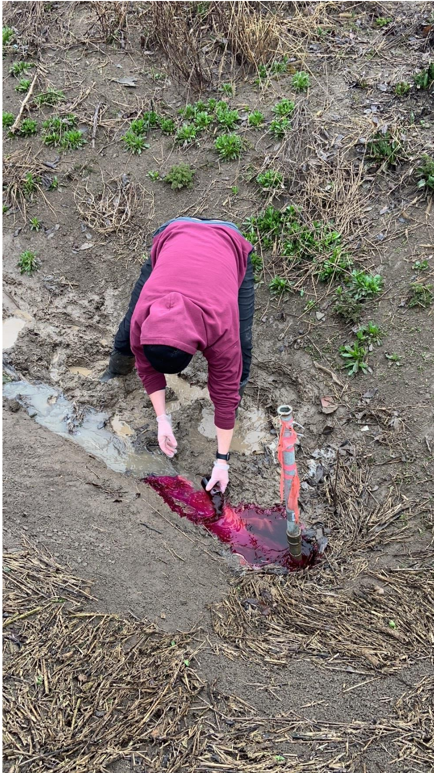
Photograph 5. Southwest view of rhodamine dye injection at SH-SE-1. 200 mL of rhodamine dye was injected at 8:32 am (Photograph was taken on April 4, 2024).
