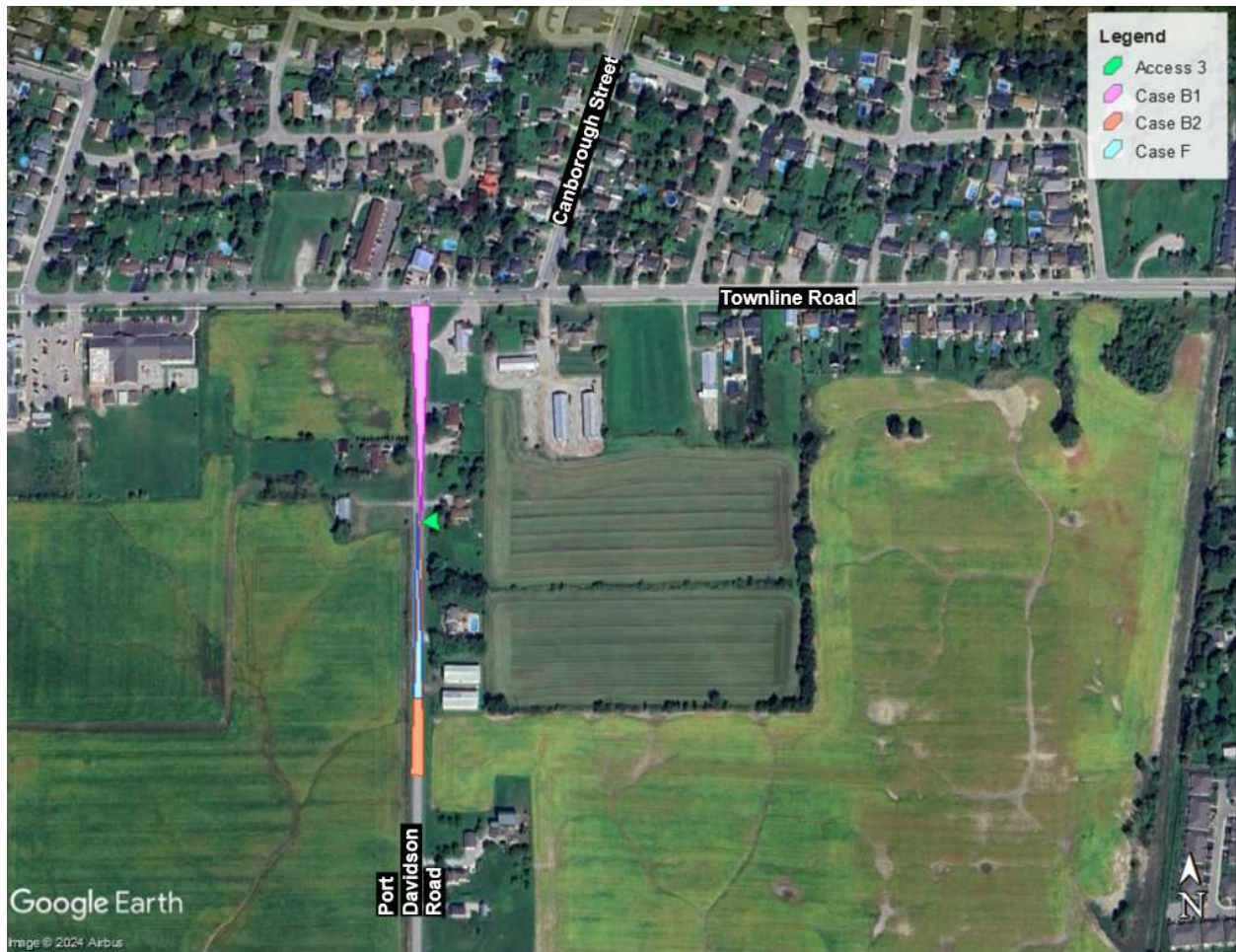
Figure 7.4: Intersection Sight Distance Requirements for Proposed Access 3
