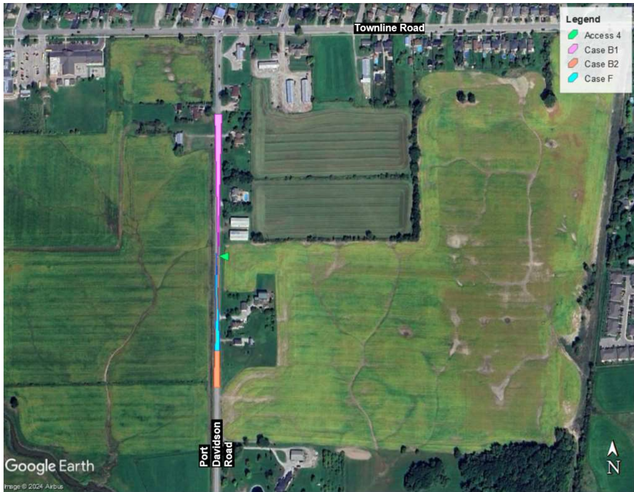
Figure 7.5: Intersection Sight Distance Requirements for Proposed Access 4
