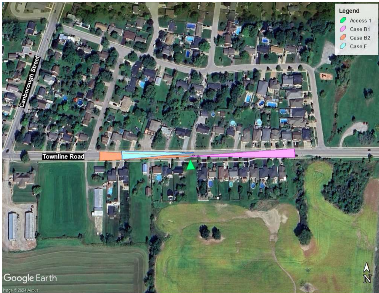
Figure 7.2: Intersection Sight Distance Requirements for Proposed Access 1
