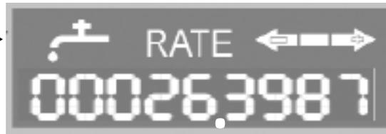
The LCD displays your reading in cubic metres. The last 4 digits to the right of the decimal are fractions of a cubic metre. An increment of 1 in the last digit to the right represents 1/10<sup>th</sup> of a litre (100mL) change. This small amount of flow indication can also be used to help confirm leaks.
