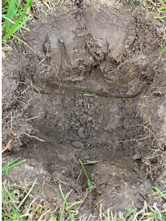
Image 19: Disturbed test pit. Very compact medium brown clay mottled with light brown and orange clay with gravel inclusions.
