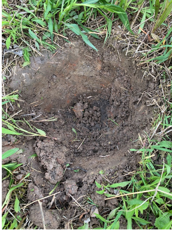
Image 17: Disturbed test pit, very compact light brown, medium brown, and orange mottled clay with gravel inclusions.
