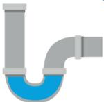
Please fill drains and rarely used sinks with one (1) pail (3-4 litres) of water on the day you receive notice or door hanger. This water in U plumbing trap will prevent the fog from entering your home.
